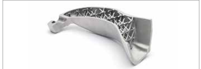
Fig. 2: Part structure with load-adapted supports
