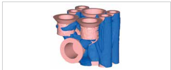
Fig. 2: Interpretation and remesh of topology optimization result
