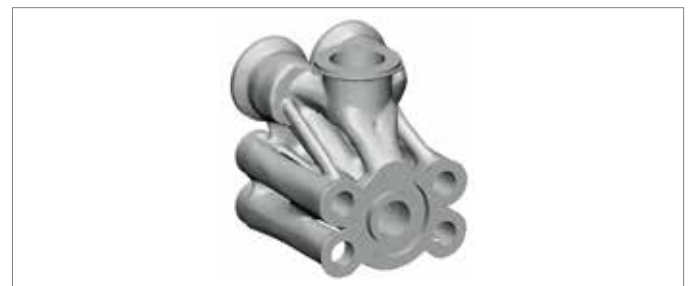
Fig. 4: Final smooth CAD file, ready for printing
